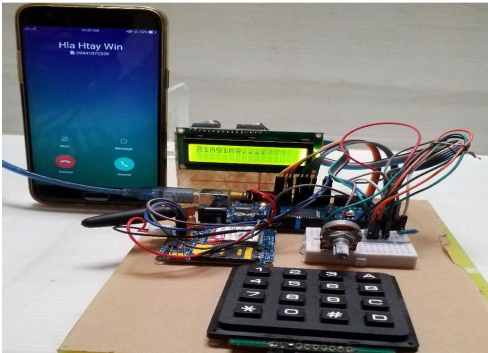
**Figure 5:** Photo of the calling the phone using GSM module
