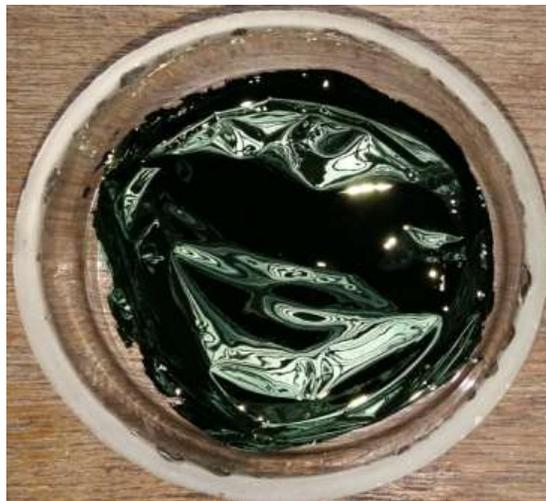
**Figure 2.** Conductive polymer film
