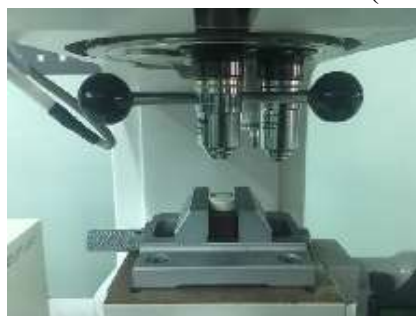
Figure 11 .Hardness measuring of F.S.HAp.-Glass Powder-GIC Composite with Mitutoyo Micro-hardness testing machine
