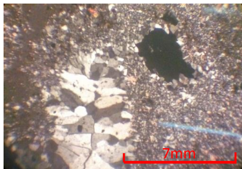
Figure 10 Chalcedonic cryptocrystalline texture, a uniform dense aggregate of cryptocrystalline quartz (Between XN)
