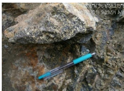
Figure 16 Impure chromite ore (Leopard ore) is less chromite content in the study area.
