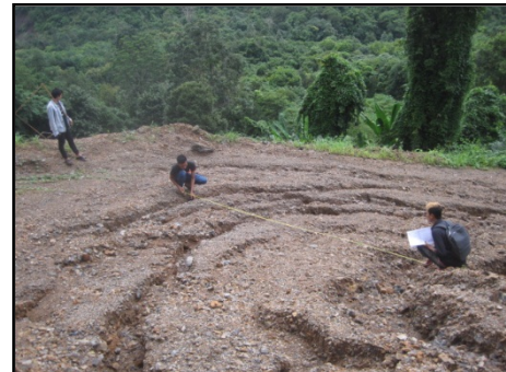
Figure 15 Creep in cherty limestone of Moulmein Limestone (N16°49' 14.6"E97°41'13.6", Facing - 80°)
