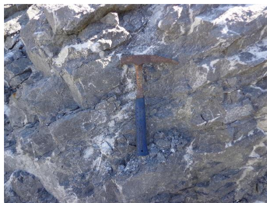
Figure 7 Grey coloured, medium- to thick-bedded, and highly-jointed dolomitic limestone, Location: 96°20'7.372" E and 22° 07' 28.425" N (Facing : East)
