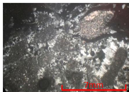
Figure 12 Crustiform texture which is successive bands oriented parallel to vein walls and defined by differences in mineralogy, or texture, colour, (Between XN)
