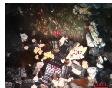
Figure 25 Quartz (Qtz), Plagioclase (Plg), Orthoclase (Ortho), Hornblende (Hb) in diorite showing allotriomorphic-granular texture (X.N)
