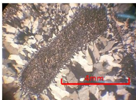
Figure 4 Cryptocrystalline variety of silica (chalcedonic quartz) filling in the cavity and lining along crystalline quartz rim. (Between XN)
