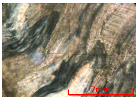
Figure 13 Moss texture: aggregate of spheroidal cryptocrystalline core and crystalline rim forming botryoidal (grape-like) texture. (Between XN)
