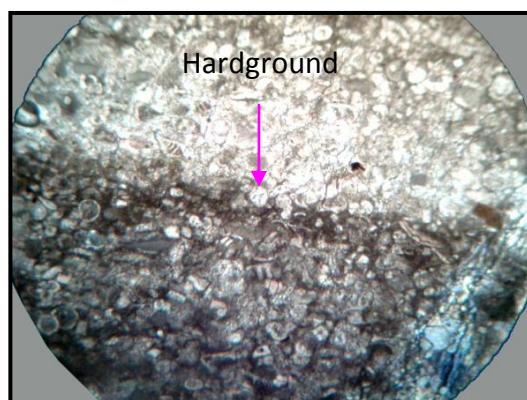
Figure 3 Photomicrographs of Globigerinid Wackestone containing Globigerinia and planar hardground with irregular surface probably formed by dissolution.
