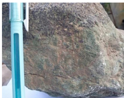
Figure 6 Serpentine (green) & chromites (black) are arranged in alternating layers.
