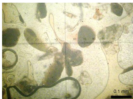
Figure10 Photomicrograph showing glauconite in fossil chamber (under PPL) (Sp. 75)
