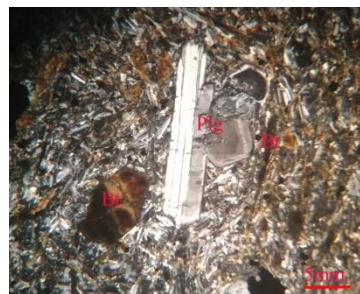
Figure 21 Andesite composed of Hornblende and Plagioclase phenocrysts (X.N)
