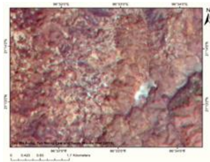
Figure 19 Alteration map by band combination of 6, 2, 1 of the study area using ASTER L1 products (cyan= alteration, brown = host rock, grey tint = gossan (Fe))
