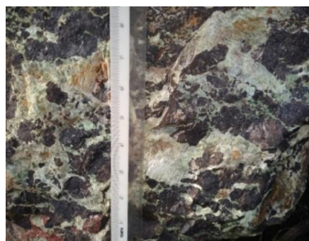
Figure 8 Nodular type chromitites consist of rounded or ellipsoidal chromite aggregates in a matrix of serpentine at Saisaquine worksite area.
