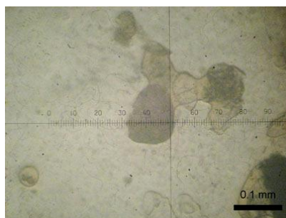
Figure 2 Photomicrograph showing glauconite grain with minute flakes (under PPL) (Sp. 63).
