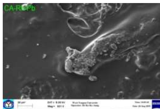
Figure 6. SEM micrographs of cellulose acetate-rice husk (CA-RH 4) composite film after lead adsorption
