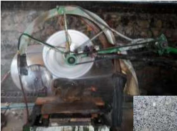
**Figure 15** Photograph shows the making of flagstones, cut off from the decorative stones.
