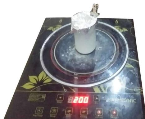
**Figure 2.** Photograph of ZnS and PVA solution by using hot plate at 80°C
