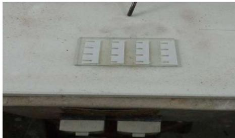
**Figure 5(b).** Heating the TiO<sub>2</sub> coated glass plate
