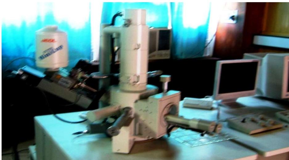
**Figure 3.** Photograph of the JEOL JSM-5610 LV Scanning Electron Microscope (SEM)
