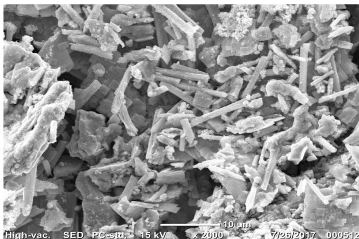
**Figure 5.** SEM image of SnO<sub>2</sub> nanorod annealing at 600°C
