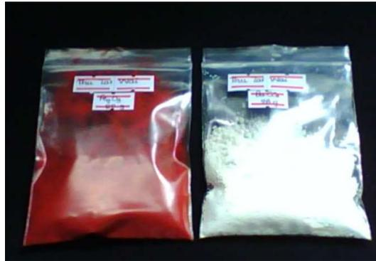
Figure 2.(a) Photograph of the weighed starting materials of Fe<sub>2</sub>O<sub>3</sub> and BaCO<sub>3</sub>
