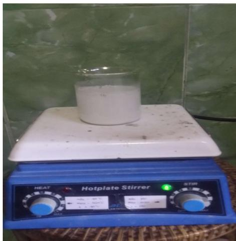
**Figure1.** Photograph of ZnS and PVA solution with magnetic stirrer
