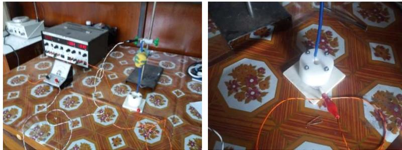
**Figure 2.** Anodization set up by single-tank Teflon holder with Pt electrode for etching small samples
