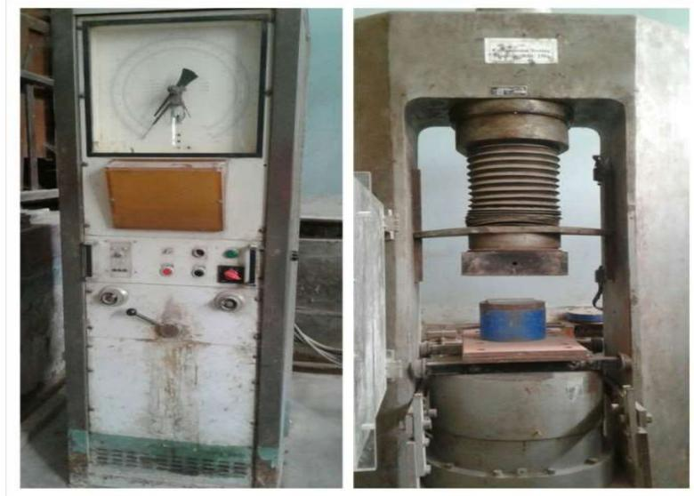
**Figure 5.** Compressive testing machine (250)
