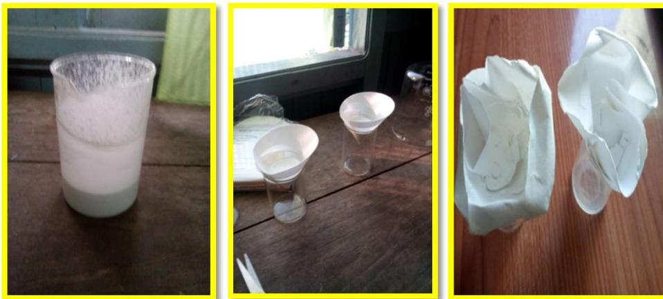
**Figure 7.** Al doped TiO<sub>2</sub> sample precipitate on flask, filter and dry in air for 120 hours
