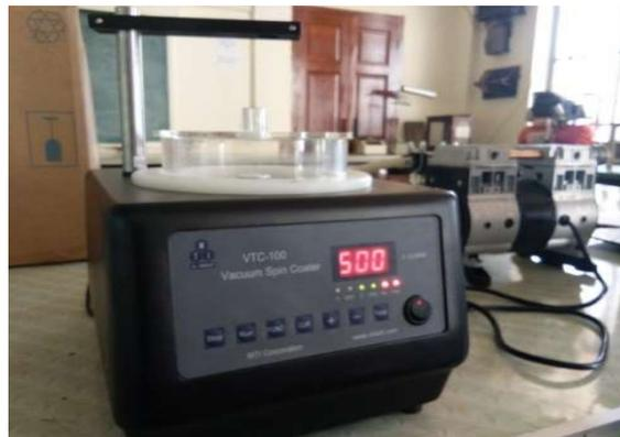
**Figure 2.** Spin Coating Machine
