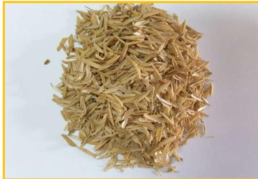
**Figure 4:** The obtained pure rice hush after doing seive analysis
