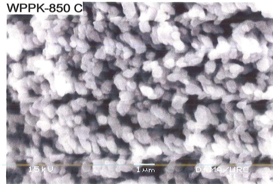
Figure 4. SEM analysis of ZnTiO<sub>3</sub> powders calcined at 850 °C
