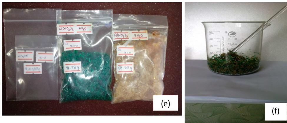
**Figure 2.** Photographs of the (e) weighed starting materials for  $x = 0.0$  sample and (f) mixed solid solutions of starting materials for  $x = 0.0$  sample
