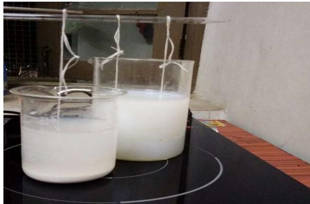
**Figure 3.** SnO<sub>2</sub>seed layer coated FTO glasses immersed into the aqueous solution
