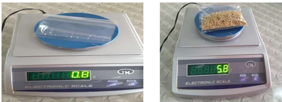
**Figure 5 :** The weight of rice husk is measured by an electronic single pan scientific balance
