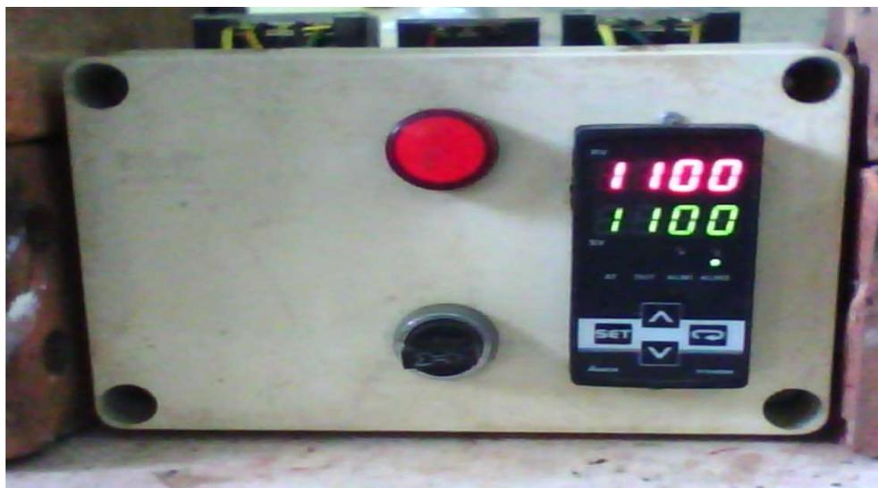
**Figure1(b).** Photograph of DELTAA SERIES DTA-4896 temperature controller
