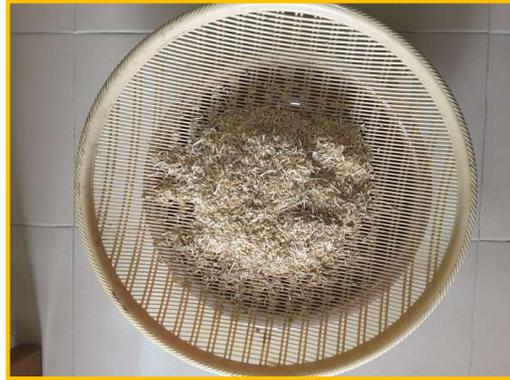
**Figure 3:** Sieve analysis of RHA using with plastic mesh
