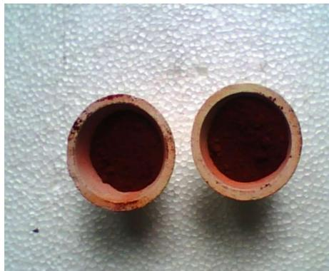
**Figure 2.(f)** Photograph of the precursor solid solution to prepare  $\text{BaFe}_2\text{O}_4$
