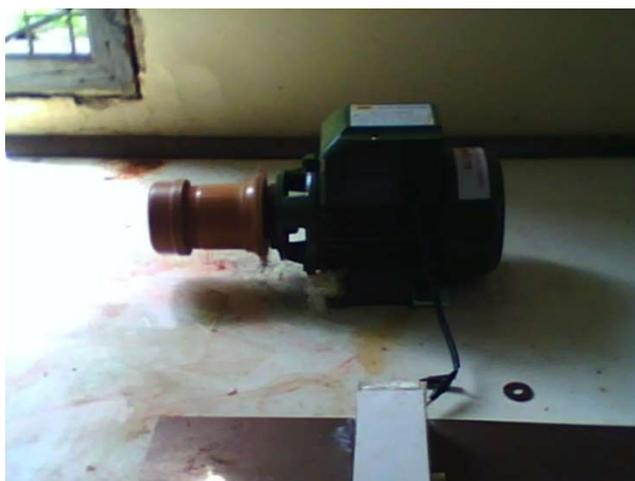
**Figure 2.(e)** Photograph of the laboratory-made ball-milling machine
