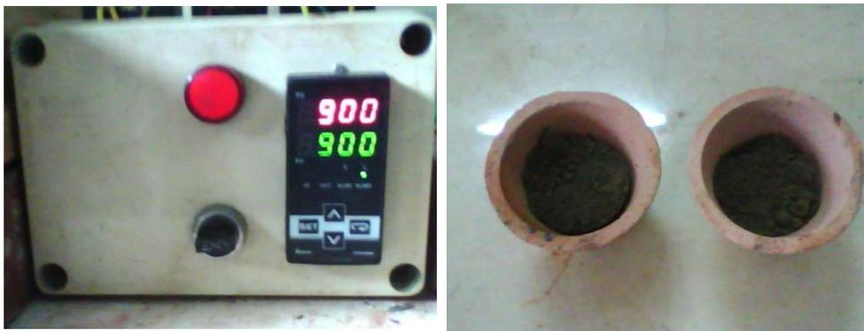
**Figure2.** Photographs of the (h) DELTA A Series Temperature Controller DTA4896 at 900°C and (i) as-prepared BaFe<sub>2</sub>O<sub>4</sub> prepared at 900°C
