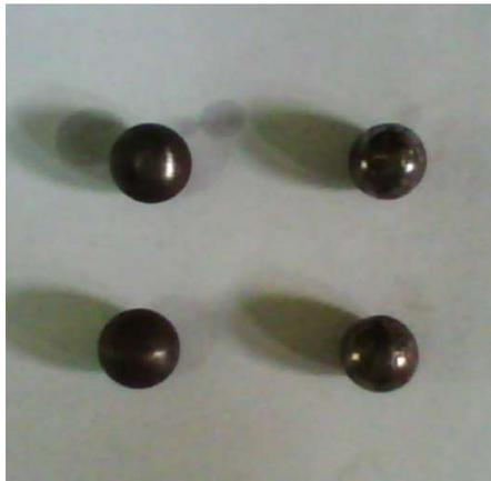
**Figure 2.(c)** Photograph of the uncoated stainless-steel ball
