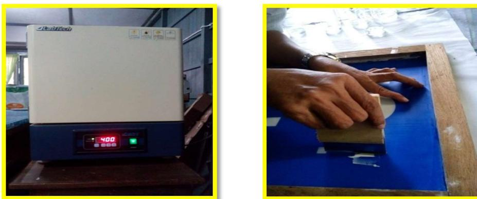
**Figure 4.** Heat treatment to mixed powder of Al and TiO<sub>2</sub>, Al doped TiO<sub>2</sub> deposited on Si and glass by screen printing method
