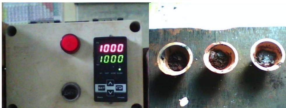
**Figure 2.** Photographs of the (l) DELTA A Series Temperature Controller DTA4896 at 1000°C and (m) as-prepared BaFe<sub>2</sub>O<sub>4</sub> prepared at 1000°C
