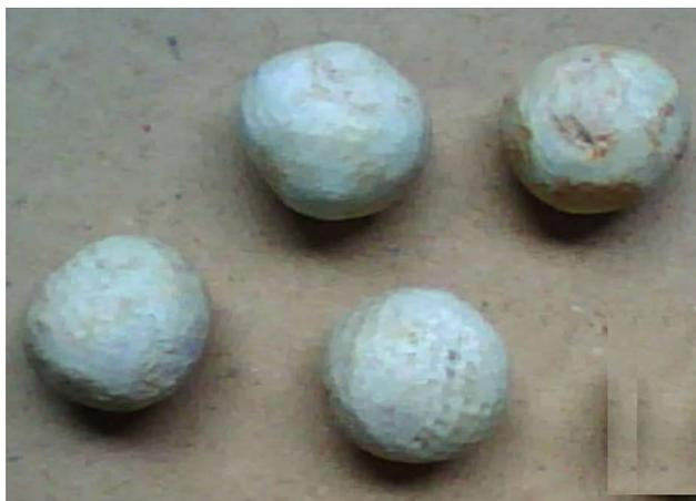
**Figure 2.(d)** Photograph of the plastic-coated stainless-steel ball
