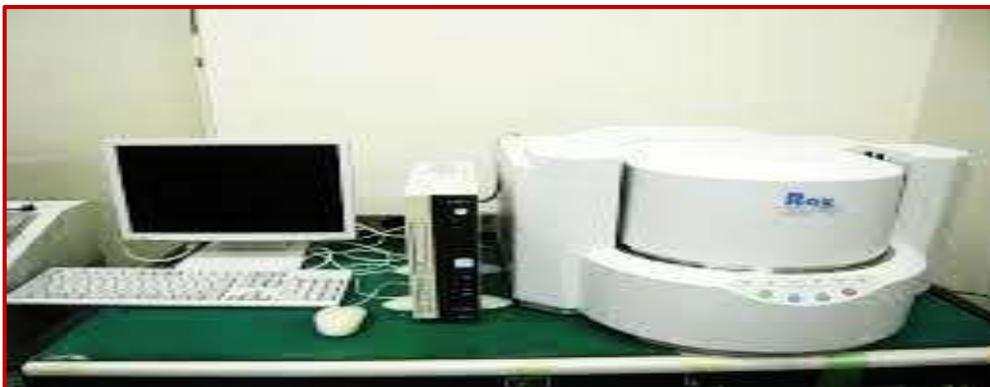
**Figure 7:** Shinmadzu EDX-720 X-ray spectrometer
