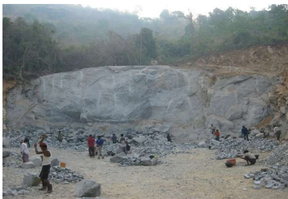
Figure 28. Biotite granite is excavated for construction and decorative stones at Daminzeik Quarry.
