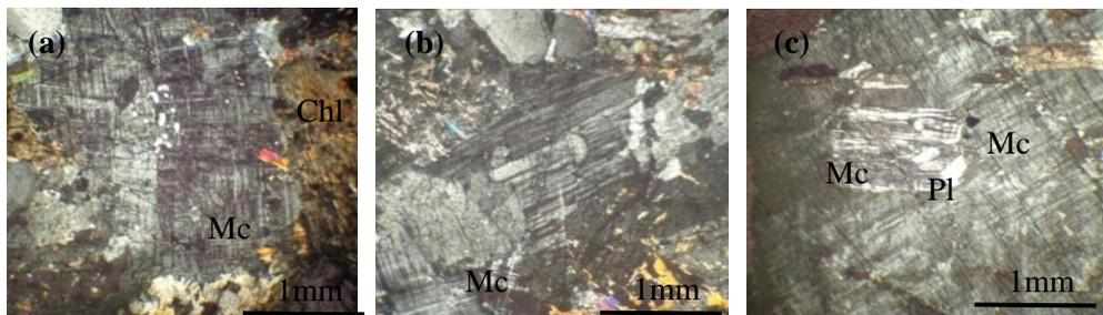
**Figure 6:** Photomicrographs showing (a) the bleb-like intergrowth of quartz in microcline and biotite altered to chlorite, (b) the microcline, perthite and plagioclase; the intensive sericitization occurs in the plagioclase and (c) microcline and plagioclase inclusions in microcline phenocryst (Mc-Microcline, Chl- Chlorite, Pl- Plagioclase)
