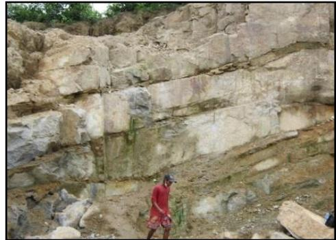
**Figure 3:** Bedded nature of porphyritic biotite granite at Banbwegon quarry ( $16^{\circ}36'20''\text{N}$  and  $97^{\circ}29'55''\text{E}$ )
