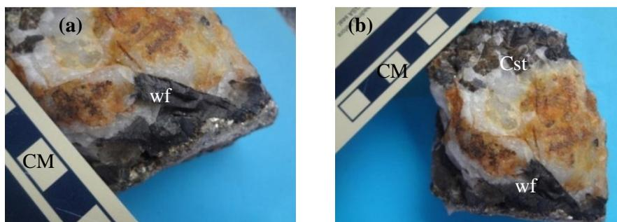
**Figure 18:** Hand specimen of wolframite and cassiterite in adit-1 of Tagu deposit
