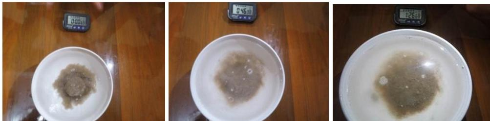
Indurated Shale (0:00 Sec) Indurated Shale (0:46 Sec) Indurated Shale (1:26 Sec)
