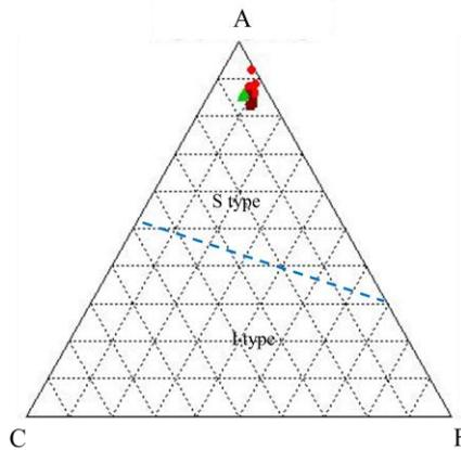
**Figure 27:** ACF diagram for the igneous rocks of the study area (after Hine et al.,1978) Molar ratio: A=Al<sub>2</sub>O<sub>3</sub>-Na<sub>2</sub>O-K<sub>2</sub>O,C=CaO, F=Fe<sub>2</sub>O<sub>3</sub> + MgO
