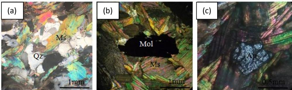
**Figure 12:** Photomicrograph showing (a) the nature of quartz and muscovite in the greisen, (b) the molybdenite with muscovite in the greisen and (c) the subhedral apatite in the greisen (Qz- quartz, Ms- muscovite, Mol- molybdenite, Ap- apatite)
