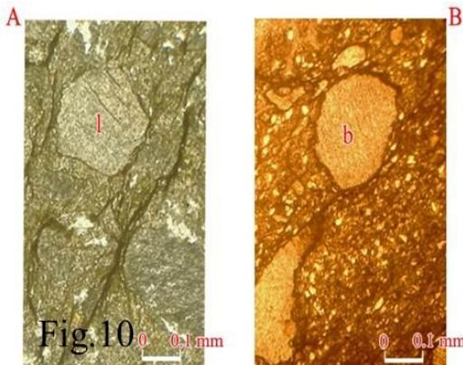
**Figure 10:** Lithoclast (l), (Fig.A) and corroded bioclastic lithoclast(b), (Fig.B) in bioclastic lithoclastic packstone microfacies. Notice that there is no grain to grain contact showing lack of deep burial compaction. PPL. (S. No. A40)
