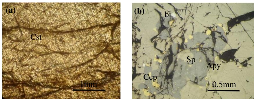
**Figure 20:** Photomicrographs showing (a) the two set of cleavage in cassiterite (under transmitted light), (b) the intergrowth texture of sphalerite and chalcopyrite; sphalerite, chalcopyrite and bismuth replaced the arsenopyrite (under reflected light) (Cst- cassiterite, Apy- arsenopyrite, Ccp- chalcopyrite, Sp- sphalerite, bi- bismuth)
