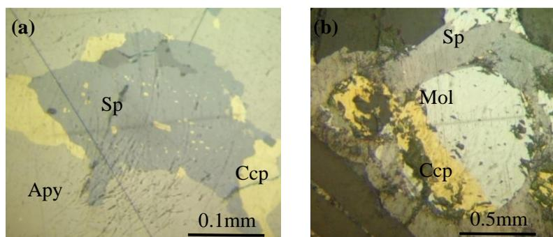
**Figure 21:** Photomicrographs showing (a) emulsion texture of the chalcopyrite and sphalerite and (b) the replacement texture of molybdenite, chalcopyrite and sphalerite in greisen (under reflected light) (Apy- Arsenopyrite, Ccp-Chalcopyrite, Sp- Sphalerite, Mol- Molybdenite)
