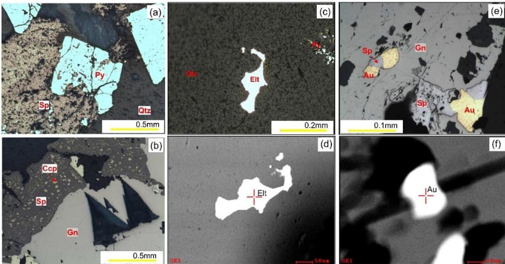
**Figure 6:** Photomicrographs showing (a) Euhedral pyrite (Py) replaced by sphalerite (Sp), (b) Galena (Gn) with triangular pits nature and chalcopyrite (Ccp) specks in sphalerite (Sp), (c & d) large electrum (Elt) grains in gold bearing quartz vein, and (e & f) fine grained native gold (Au) specks in base metals quartz carbonate vein.
