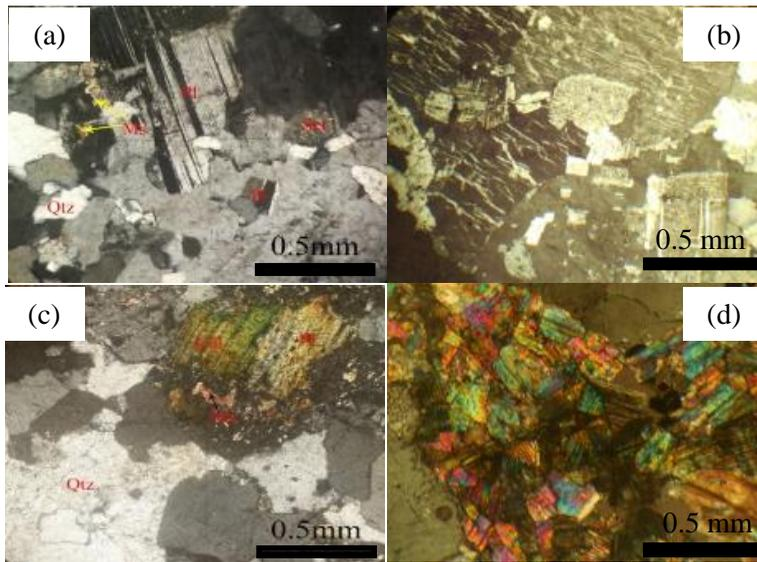
**Figure 4:** Photomicrographs showing the mineral constituent and textures of granite (a-c) and greisen (d). (a) coarse-grained plagioclase (Pl) with finer grains of quartz (Qtz) and muscovite (Ms), (b) string perthite, (c) partly chloritized (Chl) biotite (Bt) and (d) muscovite aggregate in greisen
