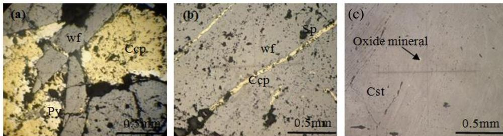
**Figure 19:** Photomicrographs showing (a) the nature of bladed, subhedral tabular wolframite replaced by chalcopyrite and pyrite, (b) the wolframite veined by chalcopyrite and replaced by disseminated sphalerite grains and (c) the oxide mineral inclusions (probably columbite) in cassiterite (under reflected light) (wf- wolframite, Ccp- chalcopyrite, Py- pyrite, Sp- sphalerite, Cst- cassiterite)
