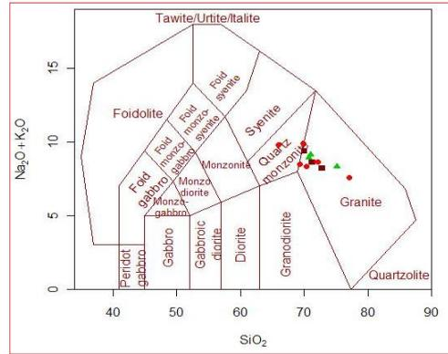
**Figure 26:** TAS diagram of Middlemost (1985) showing the Granite field of the research area
