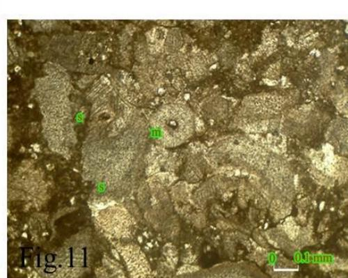
**Figure 11:** Bioclastic grains cemented by syntaxial overgrowth (s), later micritization occur. Bioclastic packstone microfacies PPL.(S.No. A.44)
