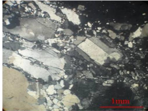
**Figure 12:** Simple twinning with orthoclase in Biotite microgranite
