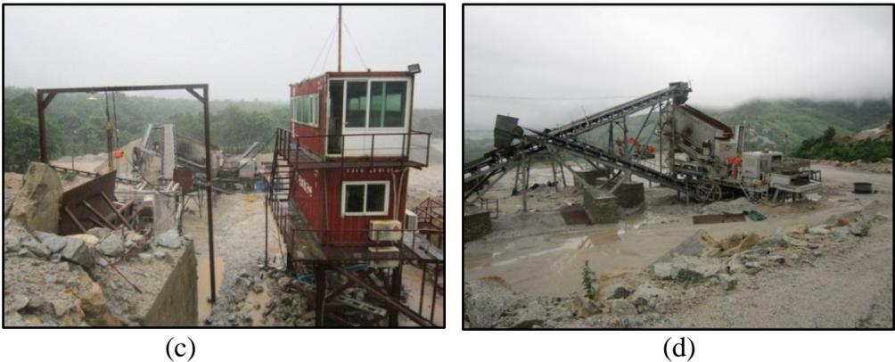
**Figure 24:** (c) Shwe Myint Mo Tun Co. Ltd., and (d) Yamanya United co. Ltd., extracting porphyritic biotite granite for construction and road materials and quality dimension slabs.
