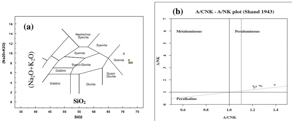
Figure 9: (a) SiO<sub>2</sub> / (Na<sub>2</sub>O+K<sub>2</sub>O) plot diagram data showing granite conditions of Tagu Taung area (Cox-Bell-Pank, 1979) and (b) Alumina saturation plot diagram showing Peraluminous nature of Tagu Taung area (Shand 1943)
