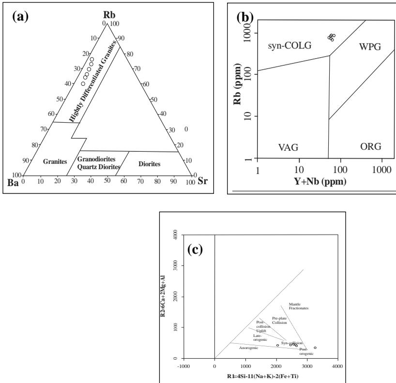
Figure 10: (a) Rb-Ba-Sr triangular plot of Tagu Taung granite (EL Bouseily and El Sokkary, 1975); (b) (Y+Nb)/Rb plot of (Pearce al, 1984) and (c) R1-R2 plot of (Batchelor and Bowden, 1985)
