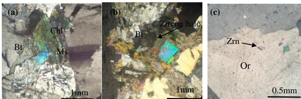
**Figure 7:** Photomicrographs showing (a) the muscovite, biotite and chlorite, (b) the zircon haloes in biotite and (c) the zircon in the orthoclase (Bt- Biotite, Ms- Muscovite, Chl- Chlorite, Zrn-Zircon)
