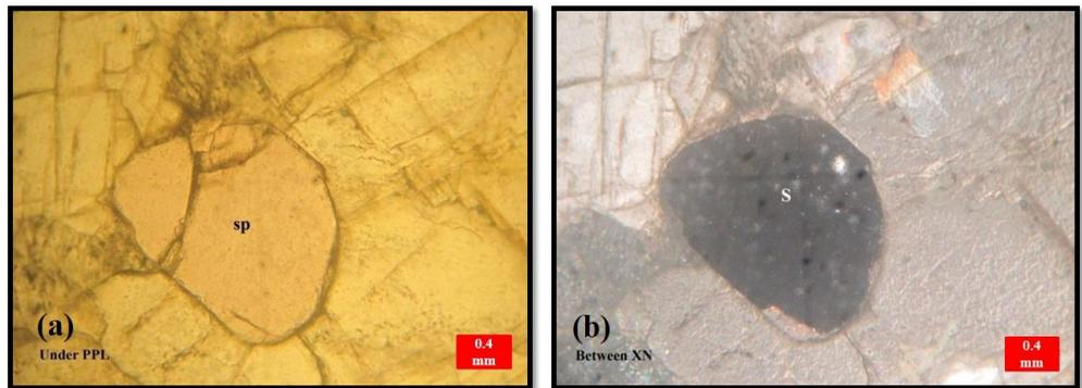
**Figure 26:** (a) (b) Photomicrograph of spinel in white marble: S= spinel
