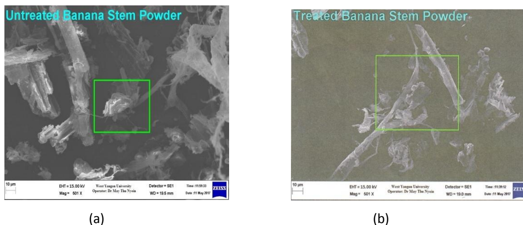
Figure 4 Scanning electron micrographs of (a) untreated banana stem fiber and (b) treated banana stem fiber (501 × magnification)
