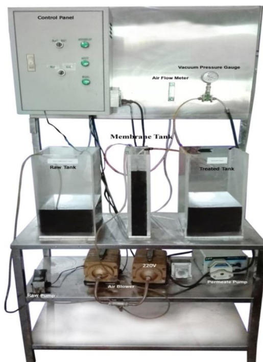
Figure 1 Treatment of Fish Sauce by Ultrafiltration Membrane Process Assembly Results
