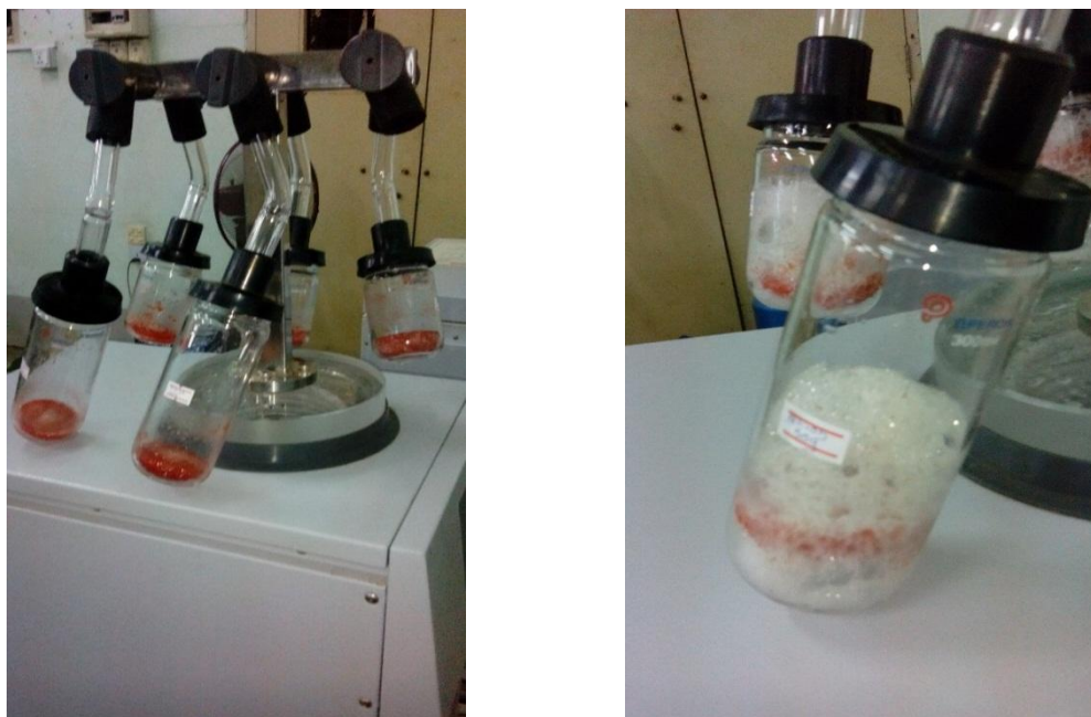
Figure 3 Preparation of Tropical Fruit Powders Using Freeze-Dryer
