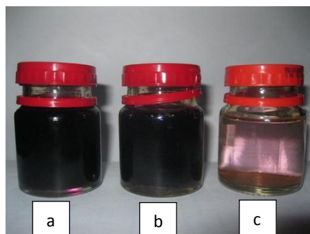
Figure 7 (a) \text{KMnO}_4 before Decolourization Decolourized \text{KMnO}_4 by Using Commercial White Charcoals from: (b) Japan (c) Myanmar
