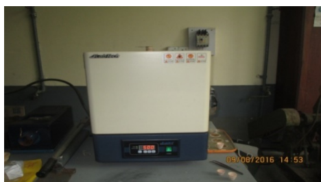
(A). Ashing samples in furnace
