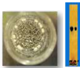
Compound 2 . (Pale yellow crystal) 2' (Authentic dihydroquercetin-7,4'-dimethyl ether) Solvent system- PE: EA (2:1) Spraying reagent -10% FeCl 3 R_f - 0.57 mpt - 165 °C
